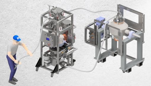
The **AM-MPRR** is jointly developed by VAC-U-MAX, Vorti-Siv and GEMCO, three American family-owned businesses with over 230 years of industrial powder handling experience. The system utilizes advanced vacuum technology to fully extract metal powders from the build box, sieves out foreign debris and oversized agglomerations, and reconditions the on-spec powder for future use.
