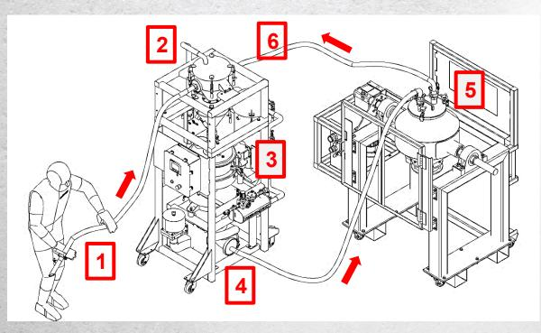
**1-2:** Operator vacuums powder from the build box which is collected in the Vacuum Receiver and is separated from the airstream by gravity. Carryover dust (if any) is collected in the small collection container on the opposite of the frame.
